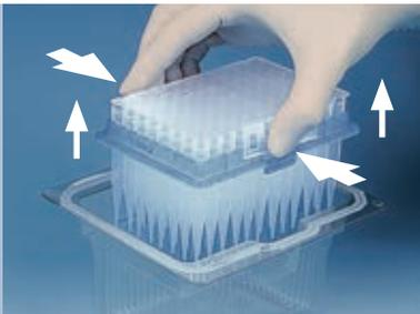
Press the long sides of the transfer aid together, and continue pressing them together while withdrawing the tip-tray. Ensure that the holding straps for the transfer aid are correctly positioned.
